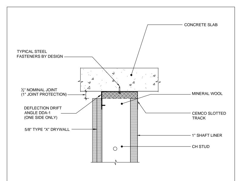
NOTE: SINGLE LAYER OF 5/8" TYPE "X" DRYWALL FOR 1 HOUR FIRE RATING
