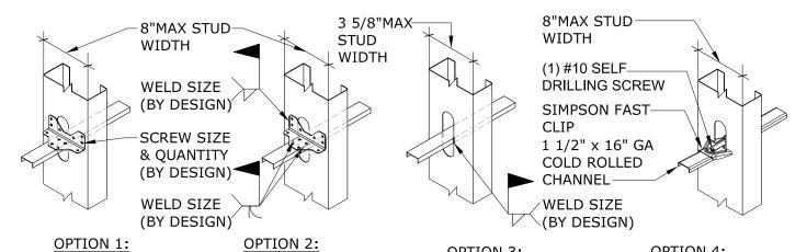
OPTION 1: SCREWED ATTACHMENT OF LATERAL BRACING
