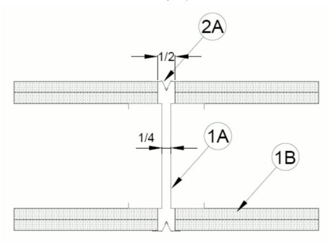
1. **Wall Assembly** — The 1 or 2 hr fire rated gypsum wallboard/steel stud wall assembly shall be constructed of the materials and in the manner described in the individual U300 or U400-Series Wall or Partition Design in the UL Fire Resistance Directory and shall include the following construction features:
