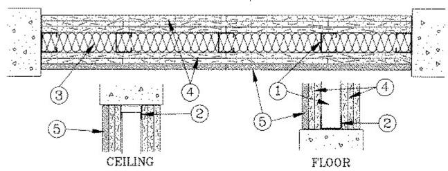
1. **Studs** — Channel-shaped, min 1-5/8 in. wide by 1-1/4 in. deep, with 5/16 in. folded back return flange legs. Fabricated from No. 25 MSG galv steel. Stud spacing not greater than 24 in. OC. Studs to be cut 1 in. less than assembly height.
