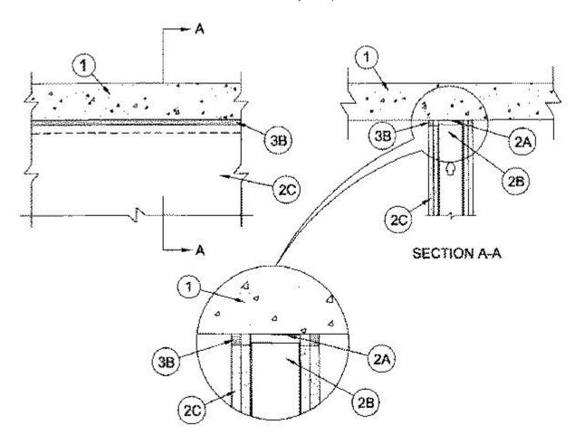
1. **Floor Assembly** — Min 4-1/2 in. (114 mm) thick steel-reinforced lightweight or normal weight (100-150 pcf or 1600-2400 kg/m<sup>3</sup>) structural concrete. Floor may also be constructed of any min 6 in. thick (152 mm) UL Classified hollow-core **Precast Concrete Units\***.
