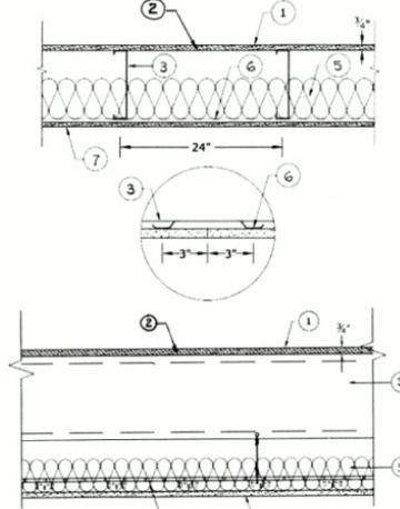
**1. Roof Covering\*** — Consisting of hot-mopped or cold-application materials which provide Class A, B or C coverings, directly applied to Structural Cement-Fiber Units(Item 2). See Roofing Materials and Systems Directory-Roof Covering Materials (TEVT).
