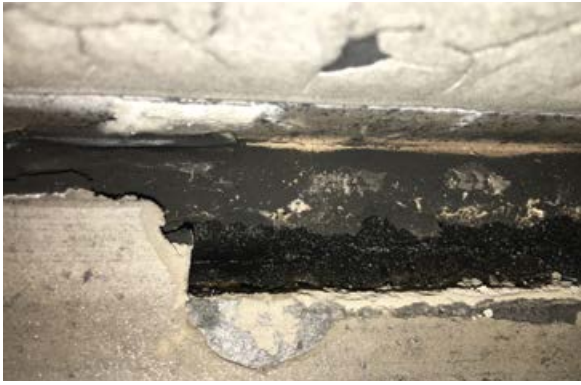
◀ Photo 3 shows HOTROD on the fire side. As shown in the photo, the intumescent material expands under fire and seals against the ceiling which prevents any smoke from passing to non-fire side.
